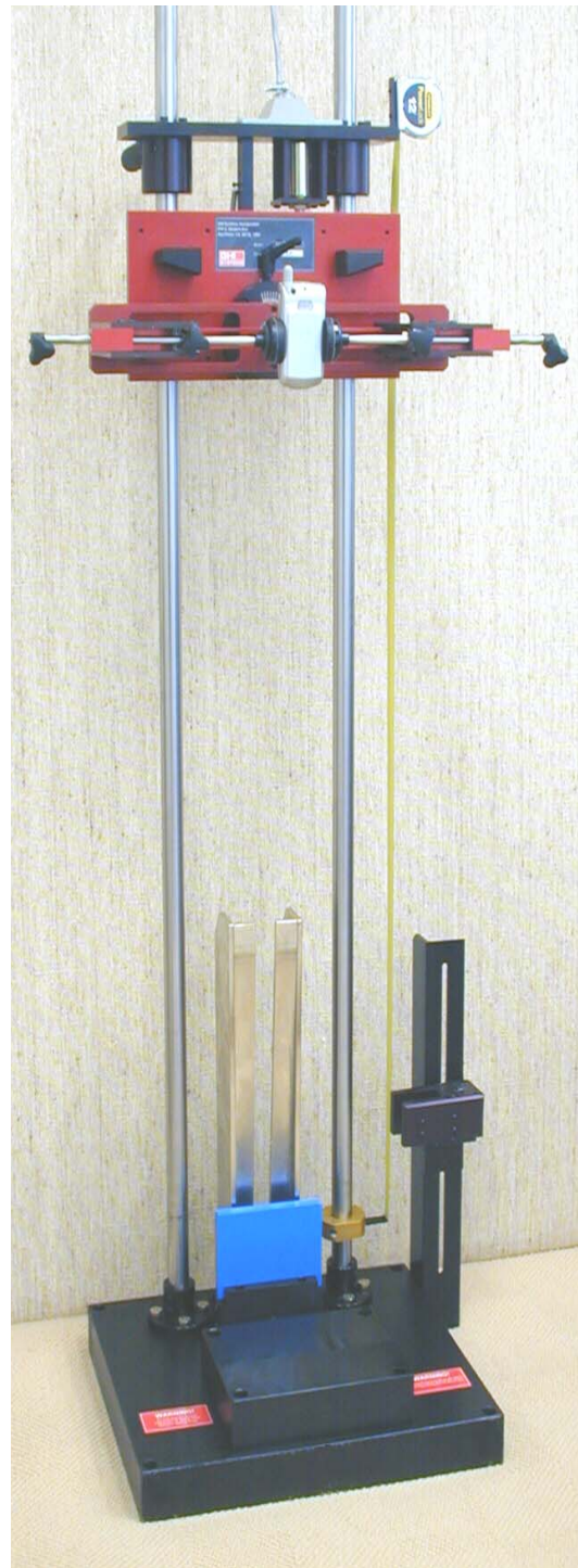
ESSM ready for a 42" drop of a cell phone onto a steel impact anvil.
